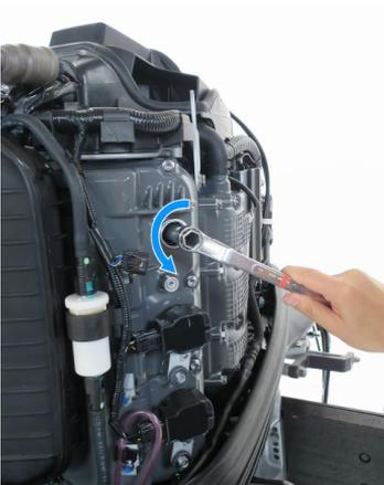
8. Remove all the ignition coil wire connectors, ignition coils and spark plugs.
