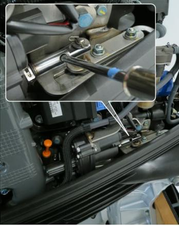
4. Insert the phillips screwdriver with the grip of the tool kit into the hole of the shift actuator.
