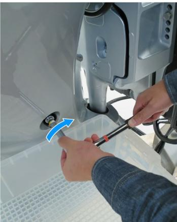
5. After draining the oil, install the drain bolt and new sealing washer, and tighten the bolt securely.
